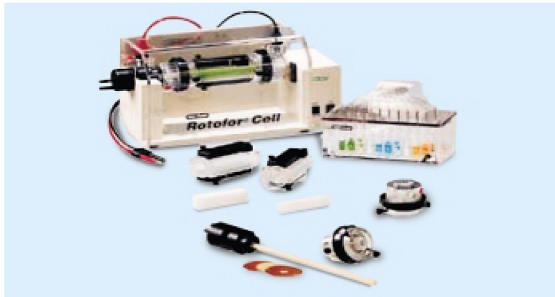
Figure 1. Rotofor apparatus with components were used to perform isoelectric focusing in liquid phase.
