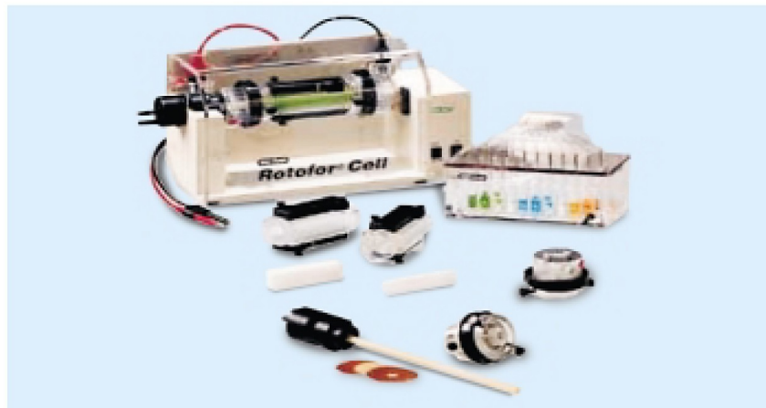
Figure 1. Rotofor apparatus with components were used to perform isoelectric focusing in liquid phase.
