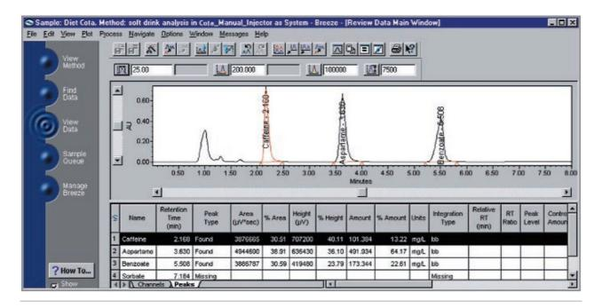
A portion of a screen capture on a Breeze System. The analysis of a diet cola shows the information that is produced together with the liquid chromatogram that the operator can examine, if desired. Note that this analysis is performed in about 6 minutes.
