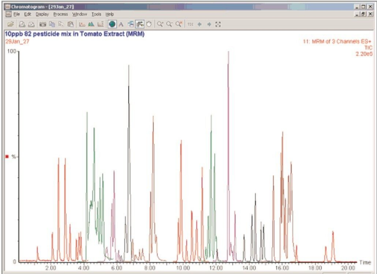
Figure 3. A chromatogram corresponding to 81 MRM functions over 11 time windows. Tomato extract spiked at 0.01 mg/kg.
