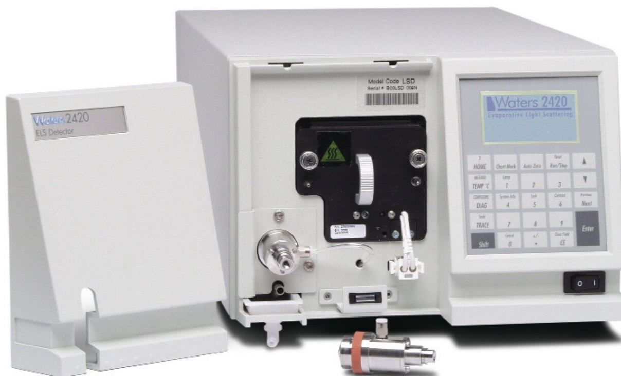
Waters 2420 Evaporative Light Scattering Detector.
