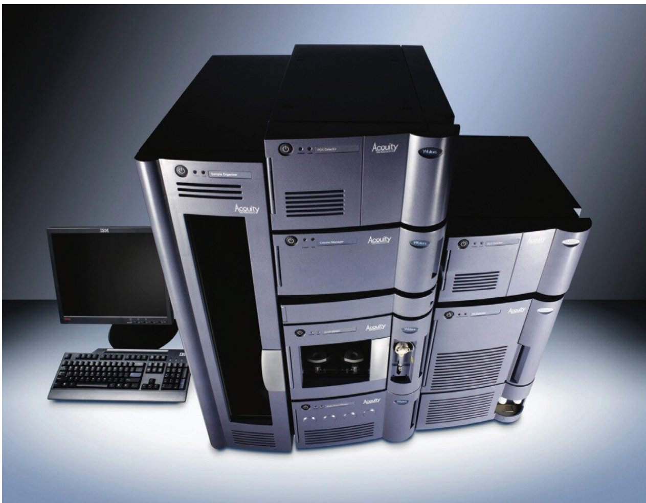
Figure 2. ACQUITY UPLC TQD System.
