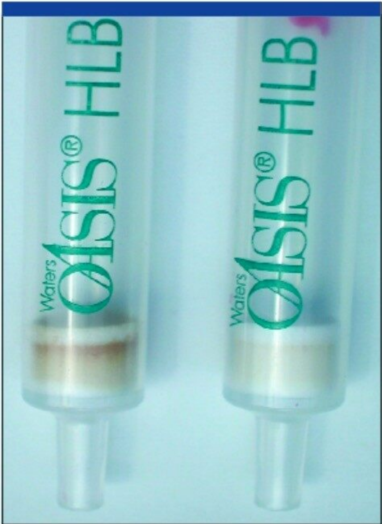
Figure 3. Left-side column (SPE Step 1): The column on the left shows the retained matrix resulting from the
