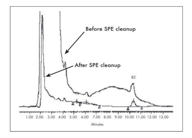
Matrix interference is greatly reduced when sample is cleaned up by using Oasis HLB SPE cartridge.
