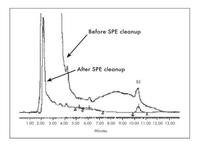
Matrix interference is greatly reduced when sample is cleaned up by using Oasis HLB SPE cartridge.
