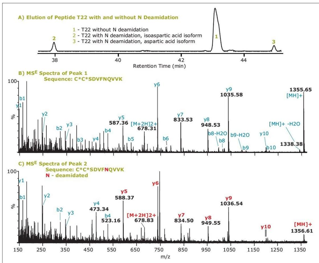
Figure 3. Elution pattern and MS<sup>E</sup> spectra of peptide T22 (C\*C\*SDVFNQVVK) without and with N282 deamidation. A) Elution pattern; B) MS<sup>E</sup> spectrum without N282 deamidation; C) MS<sup>E</sup> spectrum with N282 deamidation, isoaspartic acid isoform. y ions (marked in read) starting from y5 clearly show the deamidation. C\* is carbamidomethyl C.
