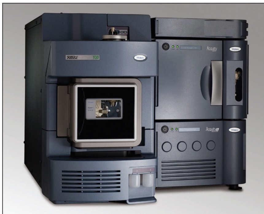
Figure 1. The ACQUITY UPLC I-Class with Xevo TQD Mass Spectrometer.
