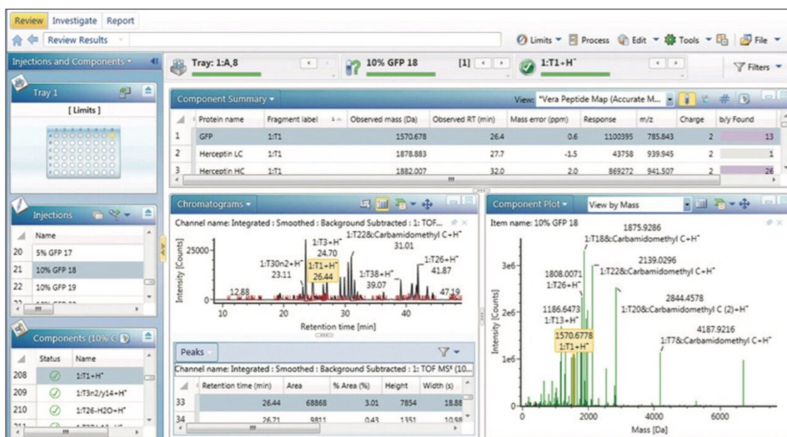
Figure 1. Processed peptide mapping data from the spiked peptide impurity study viewed within the Review tab of the Analysis Center. Highlighted within each of the sub-displays is the spiked GFP peptide.
