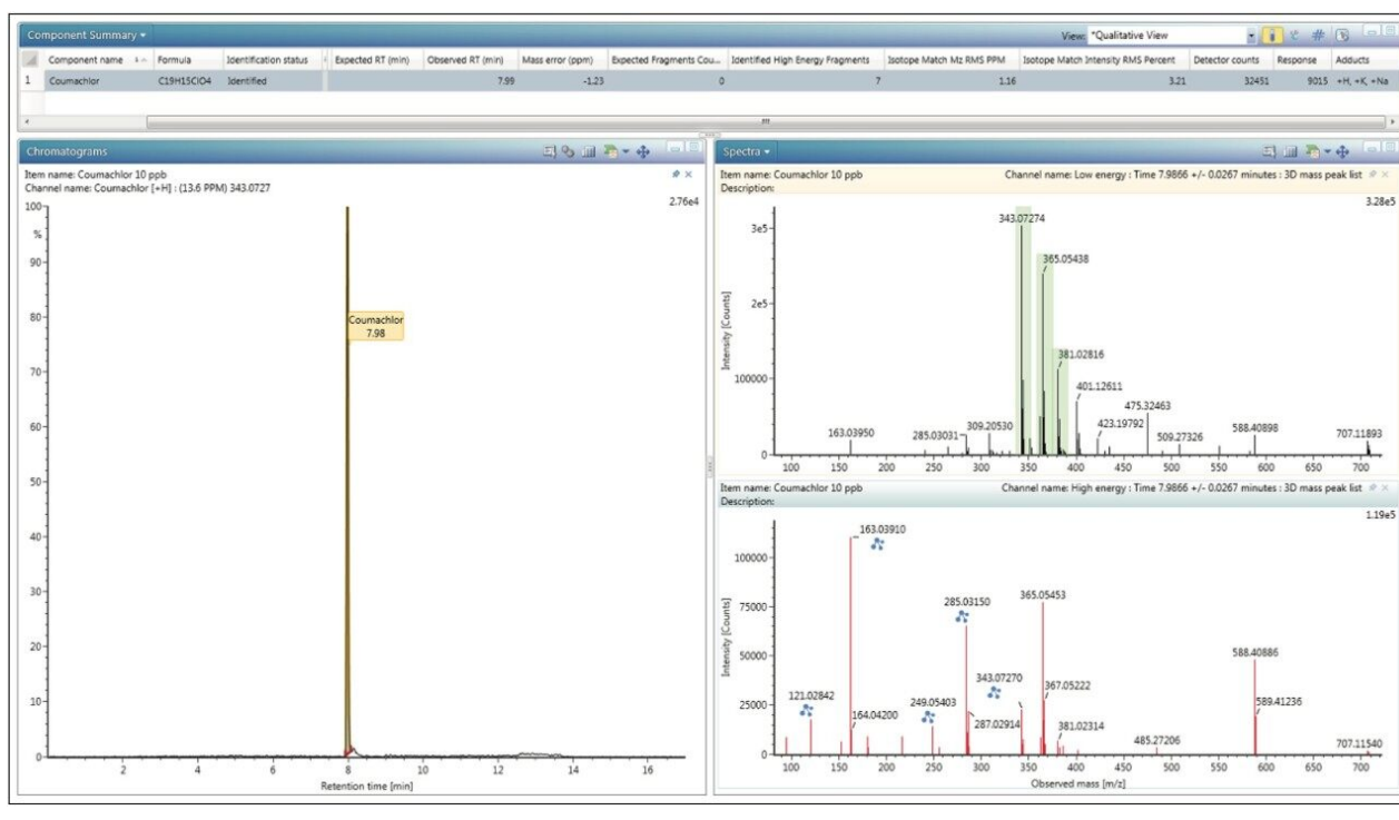
Figure 4. Coumachlor identified with accurate mass alone. Observed retention time was then added to the library. Blue icons in the high energy spectrum indicate an accurate mass product ion, automatically matched by the Fragment Match algorithm. Green area in the low energy spectrum highlight all adducts and their isotopes observed.
