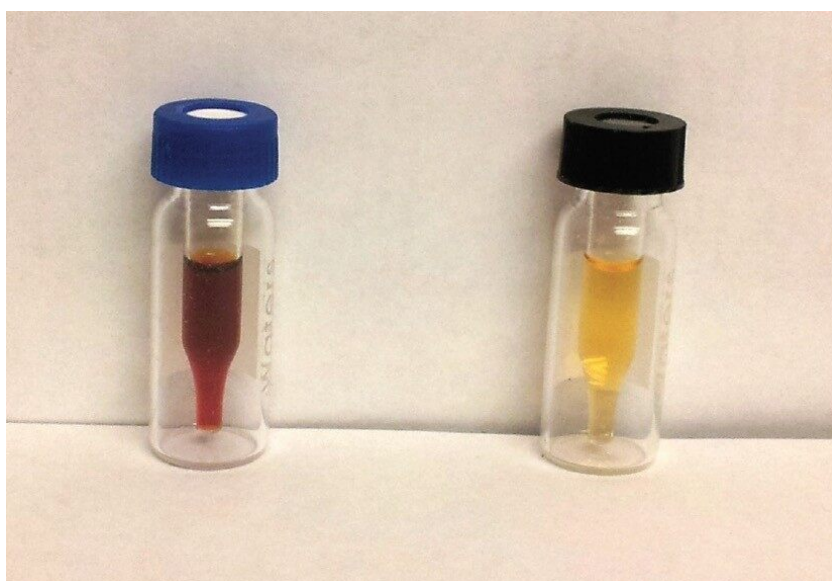
Figure 3. SPE cleanup; vial on left shows chili oleoresin sample with no cleanup, vial on right shows chili oleoresin sample after cleanup and enrichment.
