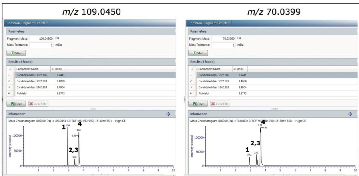
Figure 6. Common fragment search for m/z 109.0450 and 70.0399, which was used to efficiently search the technical grade flutriafol for components with common structural features.
