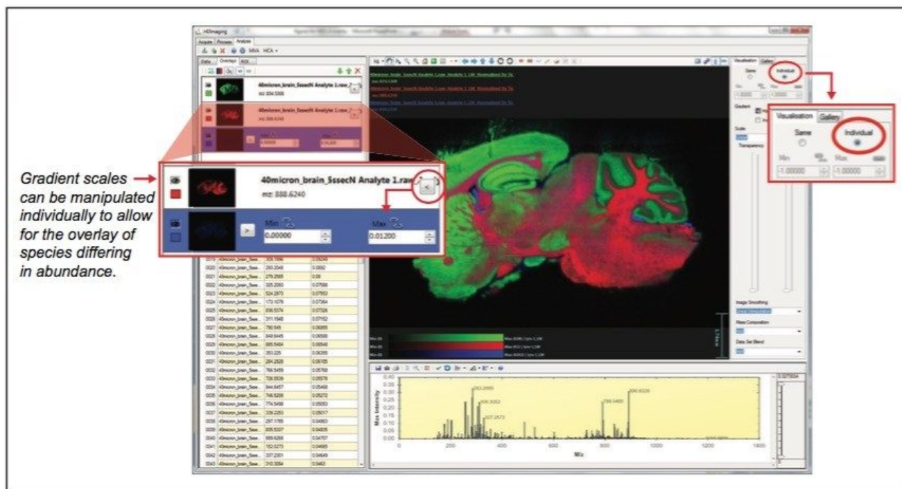
Figure 3. Generation of an RGB overlay allowing for manipulation of gradient scales combined, or on an individual basis.
