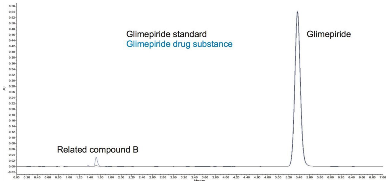
Figure 3. Overlay of standard and sample chromatograms on the Alliance HPLC system, performed using the scaled column dimensions. Blue chromatogram is the sample, black chromatogram is the standard.
