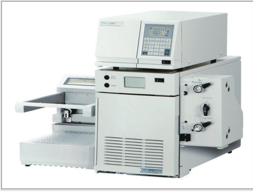
Figure 2. The Waters Prep 150 LC System.
