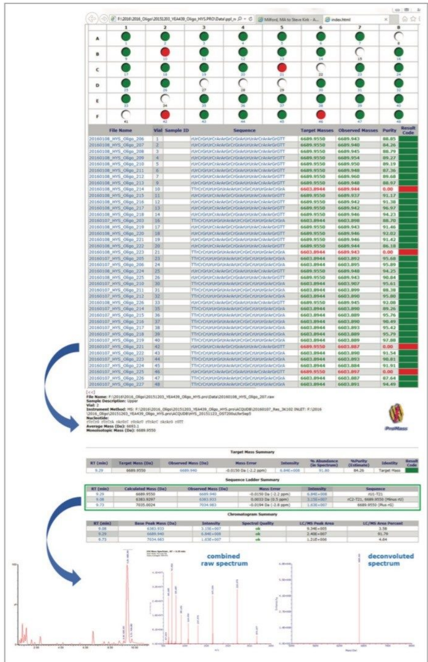
Figure 7. The top image is a high-level summary of batch-processed, experimental results using ProMass HR with MassLynx. Also shown, successive drill-down results for an individual sample, accessed through embedded HTML hyperlinks.
