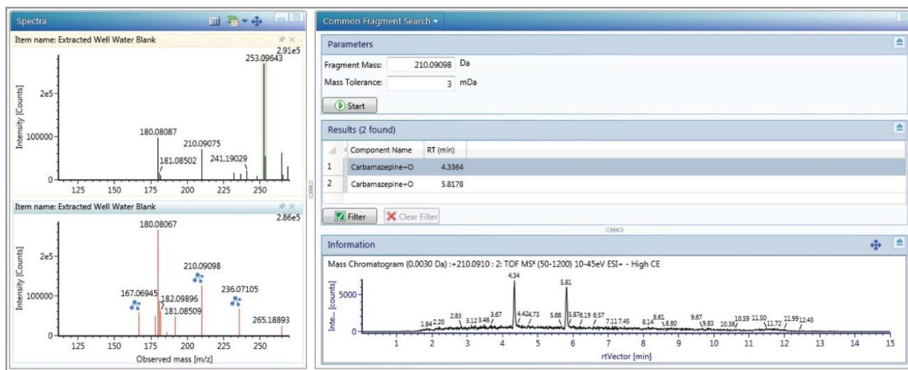
Figure 5. Results from a common fragment search of 210.09098 Da, performed within the elucidation toolset in UNIFI.
