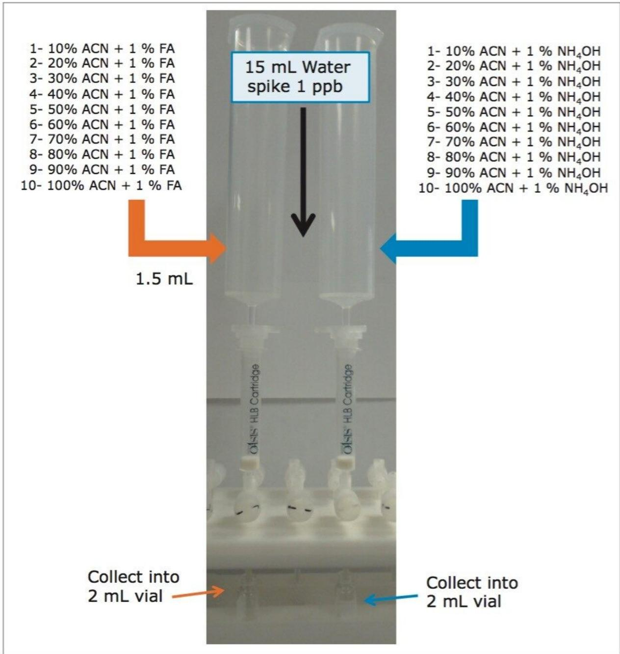
Figure 2. Sequential microextraction protocol with Oasis HLB.
