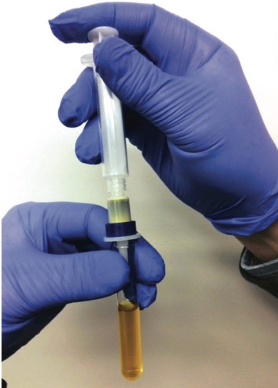
Figure 1. Oasis PRiME HLB Cartridge used in pass-through cleanup of a QuEChERS spinach extract.
