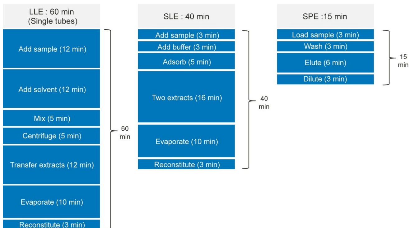
Figure 3. Protocols and processing times for LLE, SLE, and Oasis PRiME HLB extraction protocols.
