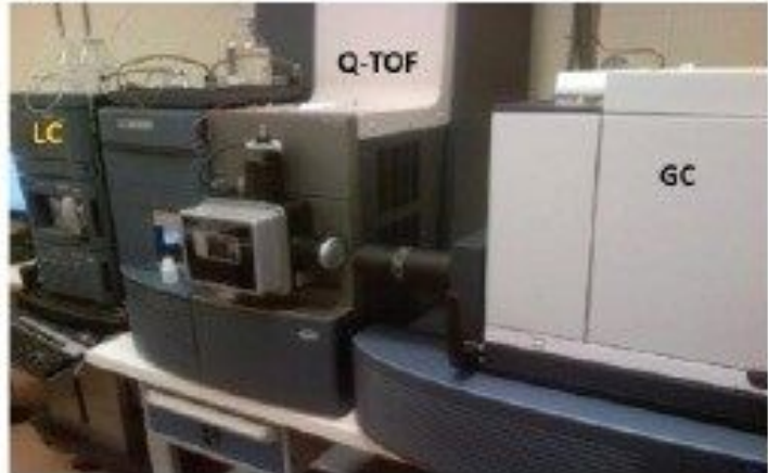
Figure 1a. Atmospheric Pressure Gas Chromatography (APGC) source on a 1b. Xevo G2-XS QToF Mass Spectrometer.
