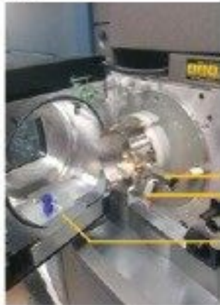
Figure 1a. Atmospheric Pressure Gas Chromatography (APGC) source on a 1b. Xevo G2-XS QToF Mass Spectrometer.
