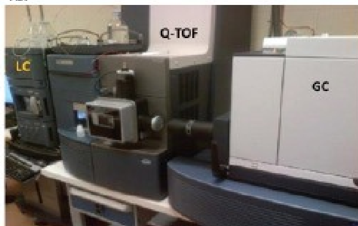
Figure 1a. Atmospheric Pressure Gas Chromatography (APGC) source on a 1b. Xevo G2-XS QToF Mass Spectrometer.
