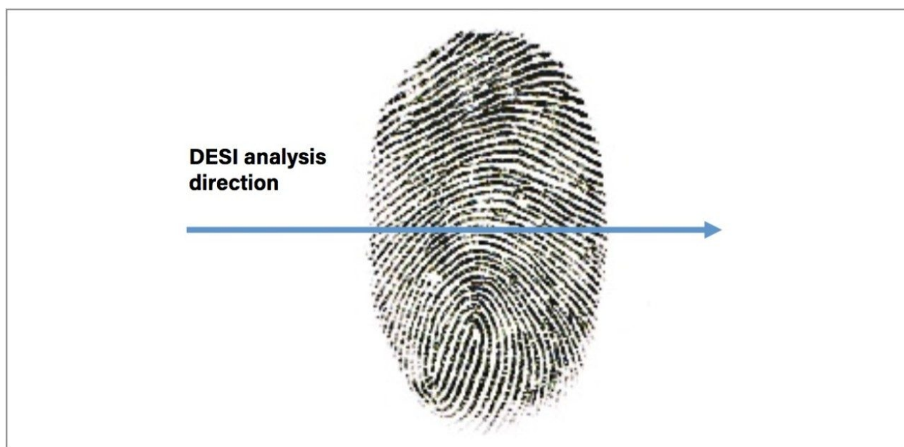
Figure 1. DESI analysis on a fingerprint deposited on a microscope glass slide.
