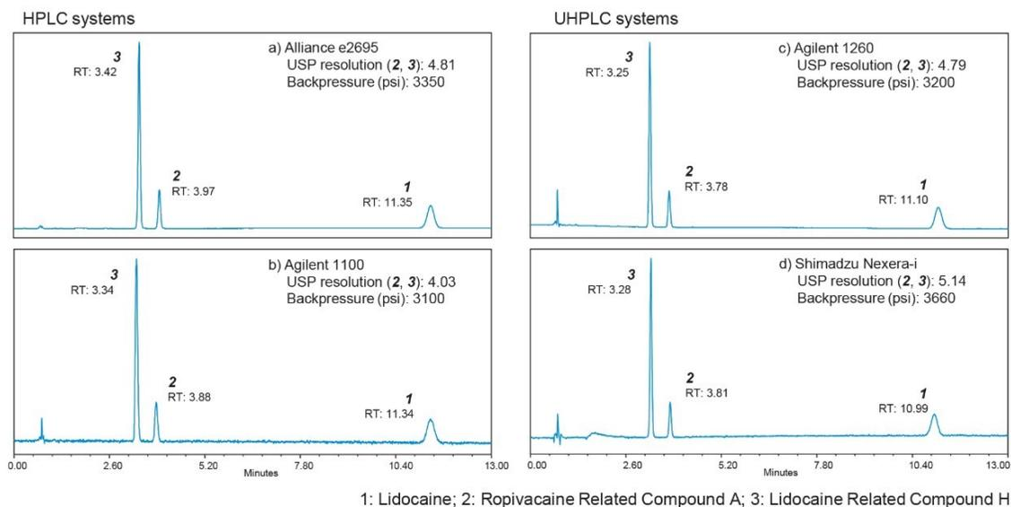
Figure 6. Chromatograms obtained on different LC instruments (HPLC and UHPLC) for the system suitability solution of the solution formulations using the XBridge BEH Shield RP18 *XP*, 2.5  $\mu$ m, 4.6 x 100 mm Column.
