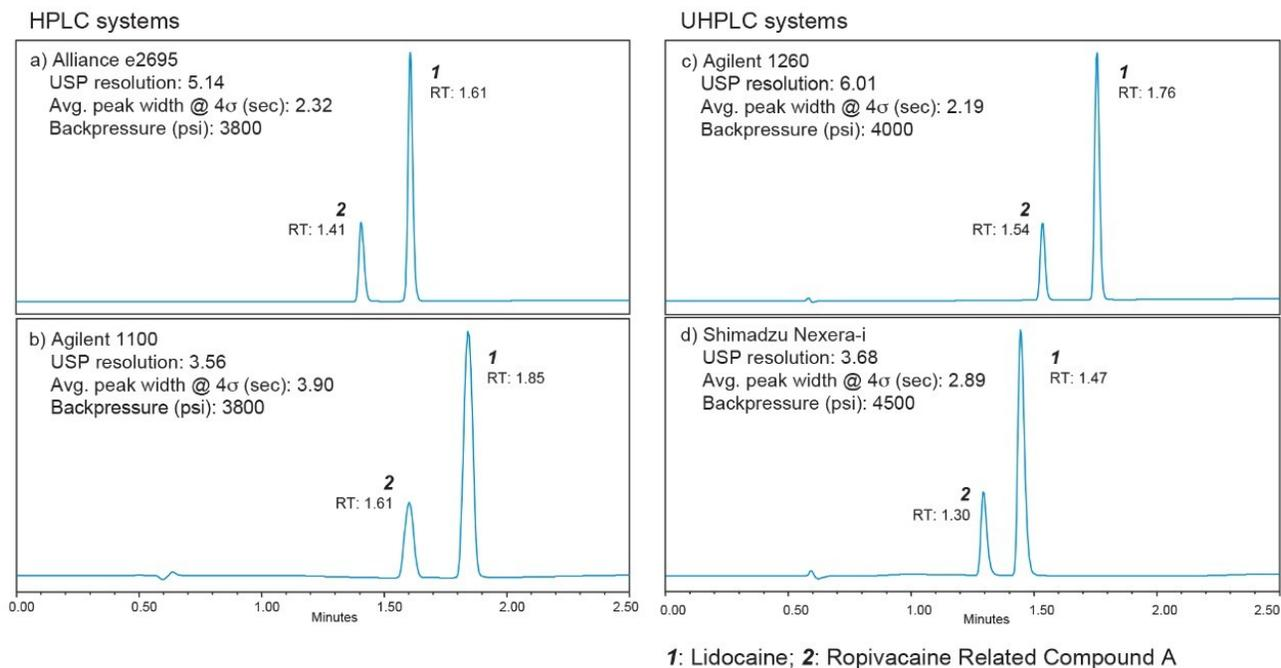
Figure 4. Chromatograms obtained on different LC instruments (HPLC and UHPLC) for the system suitability solution of the semisolid formulations using the XBridge BEH C<sub>18</sub> XP, 2.5  $\mu$ m, 4.6 x 75 mm Column.
