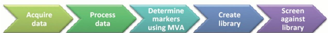
Figure 5. Workflow employed to discover differences between two lubricant oils.
