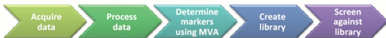
Figure 5. Workflow employed to discover differences between two lubricant oils.
