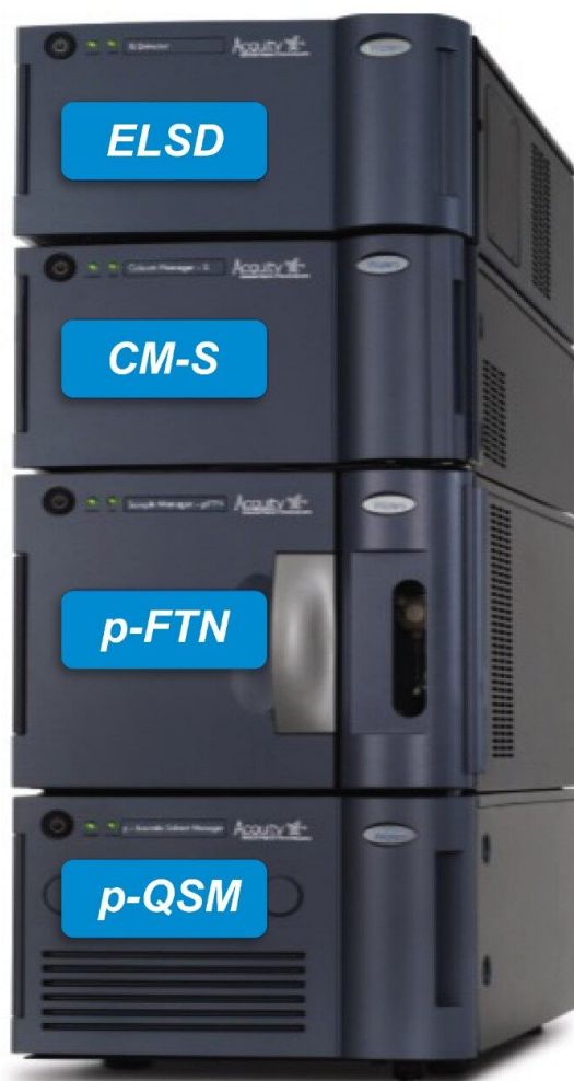
Figure 5. APC System with p-QSM and ELSD.
