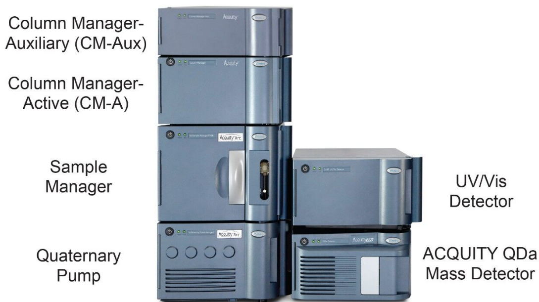
Figure 1. The ACQUITY Arc Bio System is configured with CM-A and CM-Aux column compartment modules, which can accommodate up to four 4.6 \times 150 mm columns. The CM-A module acts as the master to the auxiliary unit, and houses the valves for column selection. An ACQUITY QDa Mass Detector is configured post-optical detection.
