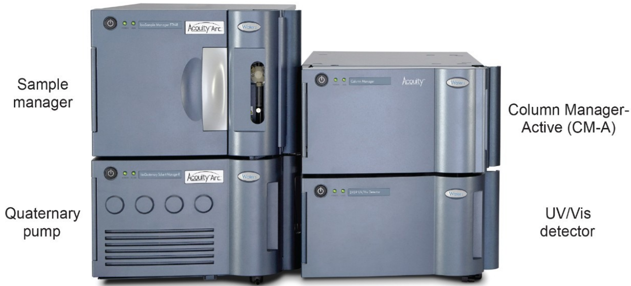
Figure 1. The ACQUITY Arc Bio System. The system is configured with a CM-A column compartment module that houses the valves for column selection between two columns. The quaternary pump enables the use of Auto-Blend Plus, which adjusts mobile phase pH and salt composition through the use of concentrated stock solutions.
