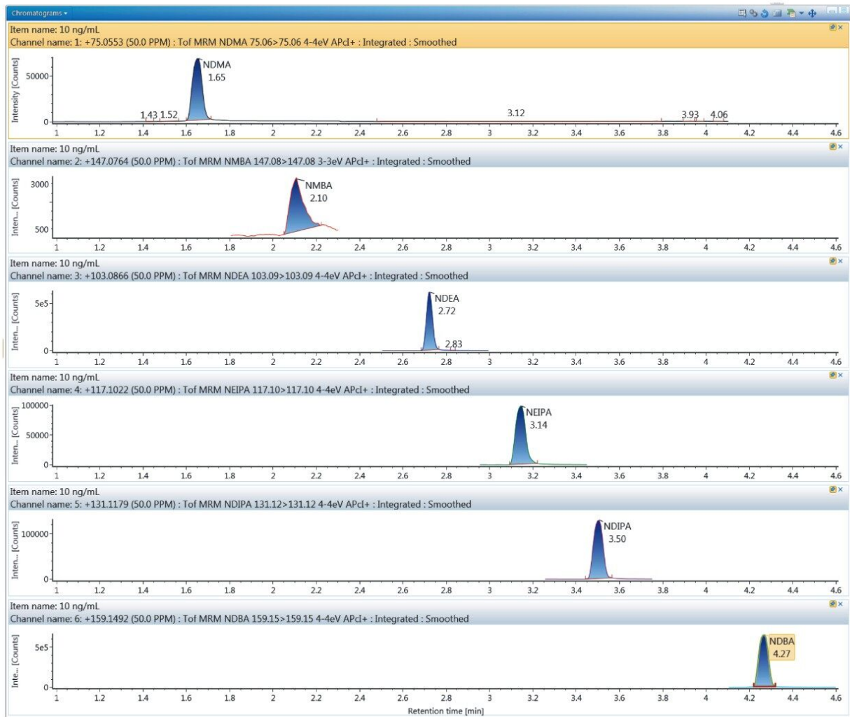
Figure 1. Extracted ion chromatograms at 10 ng/mL of all 6 nitrosamines.
