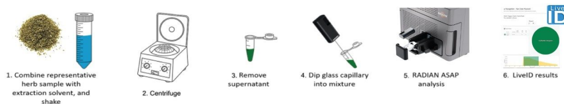
Figure 1. Illustration of the analytical workflow steps from sample dried, ground herb material to final result.
