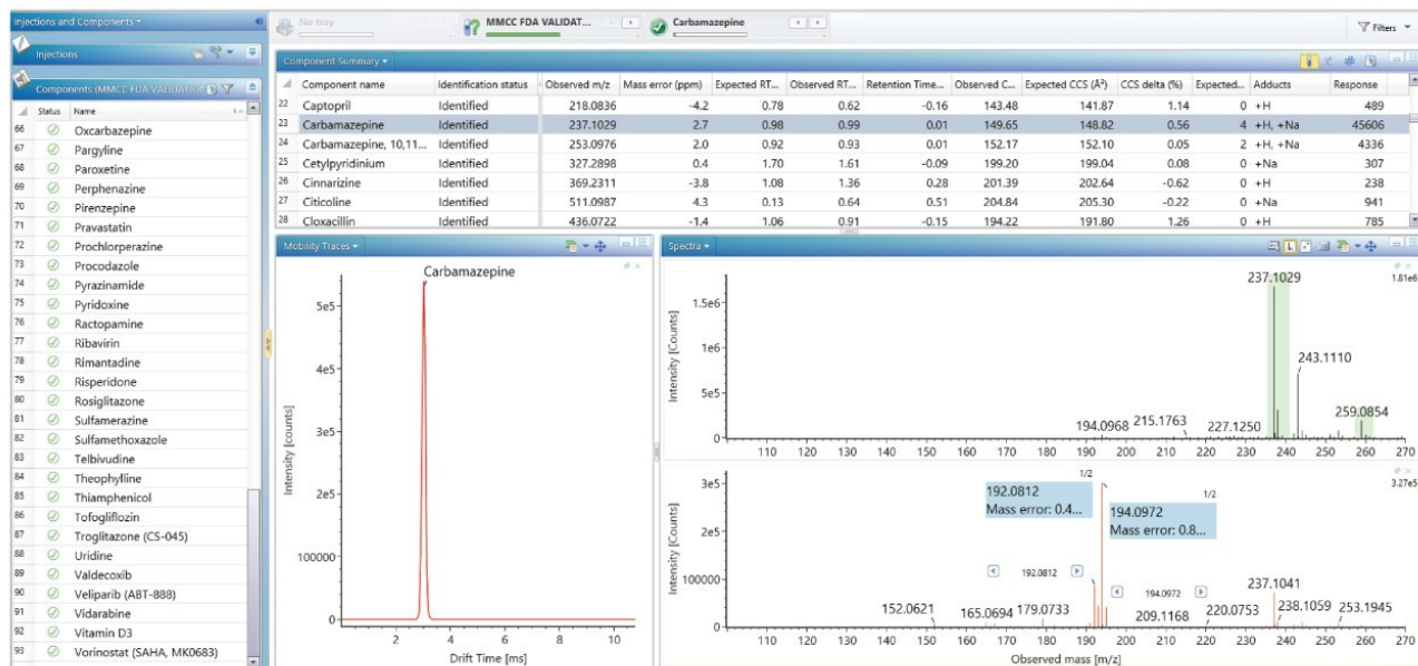
Figure 4. Post-acquisition processing workflow filtered detection results (identified count 93) for screening against 1285 FDA approved drug small molecule library, applied t_r tolerance 2.0 min, mass accuracy \pm 5 ppm, and \Delta CCS < 2\% .
