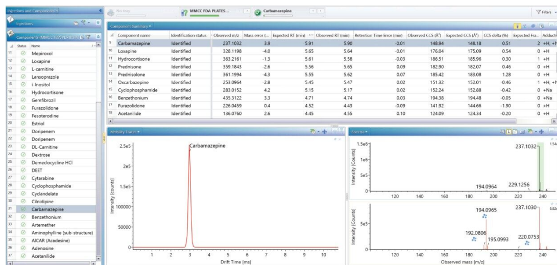
Figure 3. Post-acquisition processing workflow filtered detection results (identified count 37) for screening against FDA approved drug small molecule library, applied tolerance t_r 0.1 min, and mass accuracy \pm 5 ppm and \Delta CCS < 2%.
