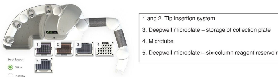
Figure 2. Andrew+ Deck layout for sample preparation of EtG and EtS in human urine using Andrew+ pipettes for pipette mixing.
