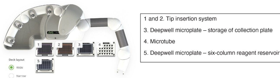
Figure 2. Andrew+ Deck layout for sample preparation of EtG and EtS in human urine using Andrew+ pipettes for pipette mixing.
