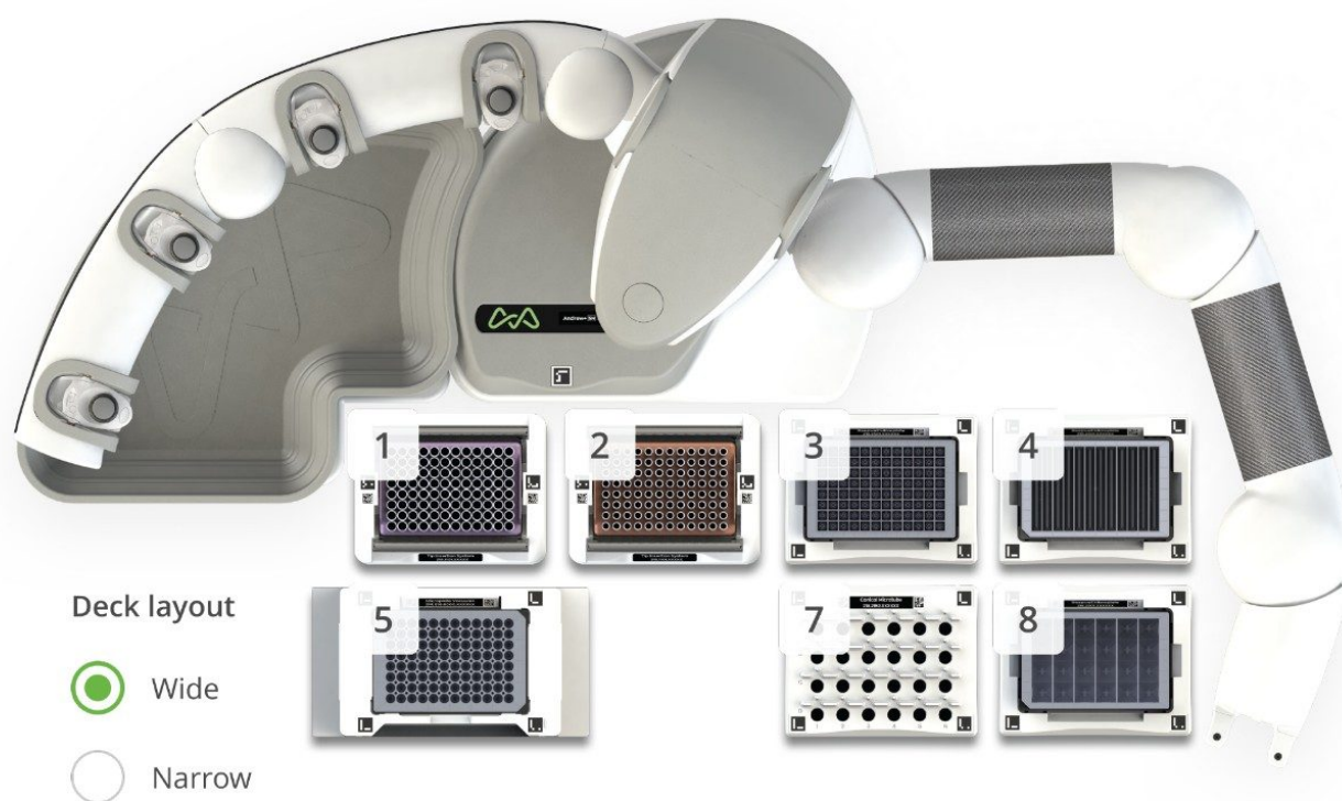
Figure 1. Andrew+ MMA Deck configuration – Dominos: 1 and 2: Tip insertion system; 3,4, and 8: Deepwell microplate; 5-: Microelution Plate Vacuum+; 7: Microtube.
