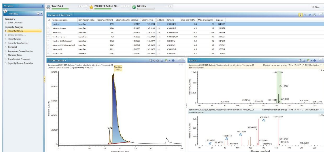
Figure 10. Identification of related impurities of Nicotine API by using transformations tool and incorporating the impurity analysis UNIFI workflow.
