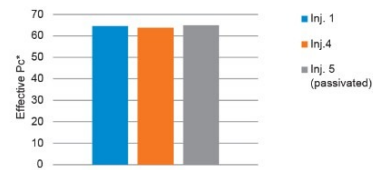
Figure 2. Impact of column conditioning on HILIC of N-Glycans when using ACQUITY Premier Columns.
