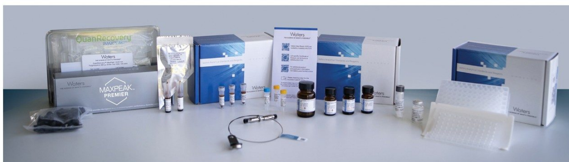
Figure 1. The SARS-CoV-2 LC-MS Starter Kit (RUO) for the analysis of SARS-CoV-2 NCAP peptides using LC-MS/MS.
