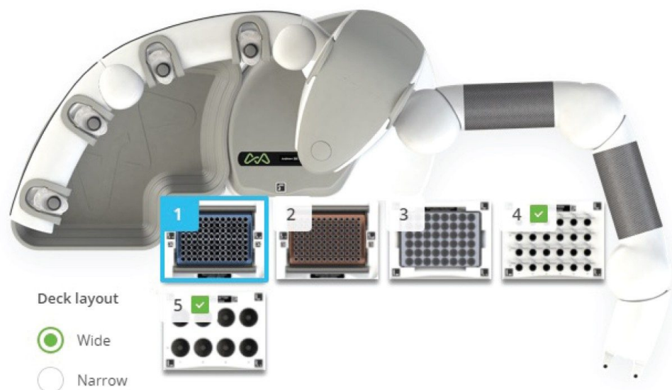
Figure 3. Schematic of the Andrew+ robot showing the positioning of each domino and the content required for the protocol selected.
