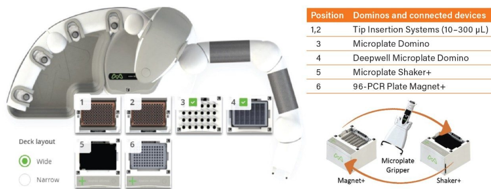
Figure 4. Andrew+ Dominos and Connected Devices configuration for the rapid automated antibody purification eight-sample protocol. For a fully automated protocol, Andrew+ requires two connected devices (Magnet+ and Shaker+) and a microplate gripper or a microplate grabber. The execution time for eight samples is 35 min.
