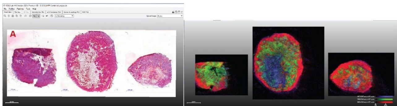
Figure 4. Displaying multiple ion distributions as a RGB overlay for multiple samples in the same project ( m/z 885.6 (red), 700.5 (green), and 687.6 (blue)).
