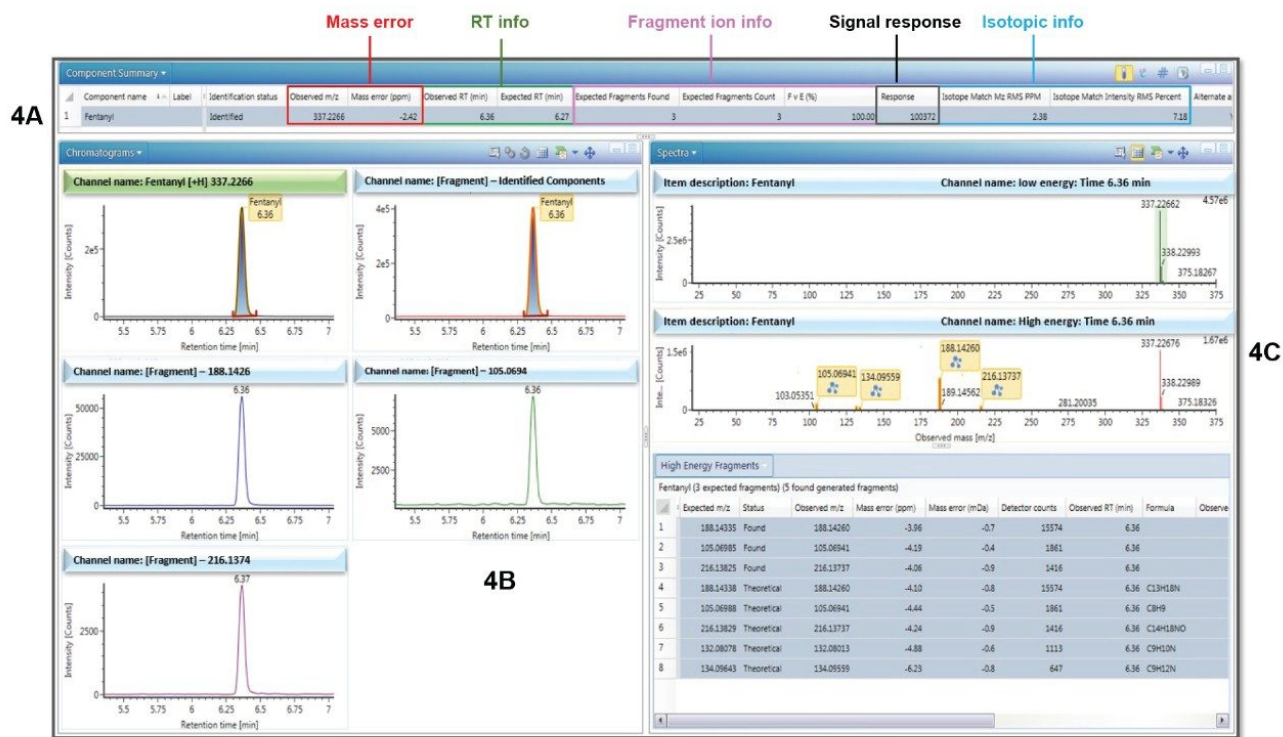
Figure 4. Detection of fentanyl in a sample following targeted analysis. A wealth of information is available and may be viewed if desired. In this figure the upper table (4A) details the results of the comparison of acquired data against the reference information contained in the Toxicology Library. Panel 4B displays the extracted ion chromatograms for the targeted precursor and the 3 diagnostic fragment ions and demonstrates that all ions are time-aligned at 6.36 min. The low and high energy spectra are shown in Panel 4C (upper). Details of the fragment ions are listed in the lower table.
