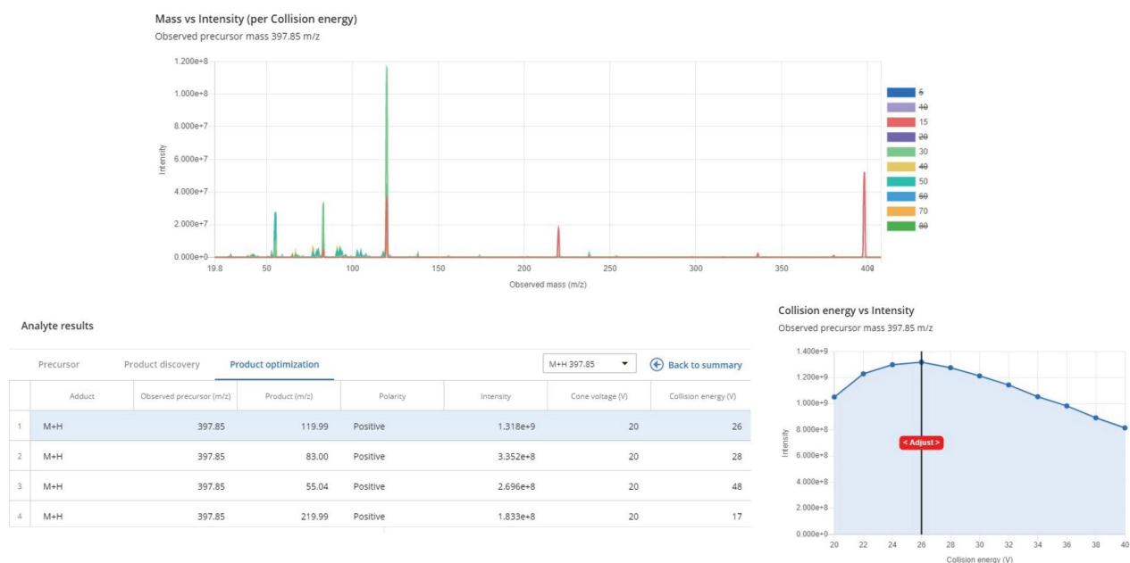
Figure 2. Example of Optimization tool output: mass spectrum of Echimidine as a function of collision energy (top), table with first 4 optimized product ions (bottom left), interactive collision energy plot for product ion m/z 120 (bottom right).
