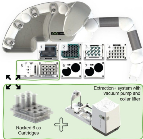
Figure 6. Andrew+ configured with Extraction+ with protocol visualization, system components identification, and Andrew+ deck layout.
