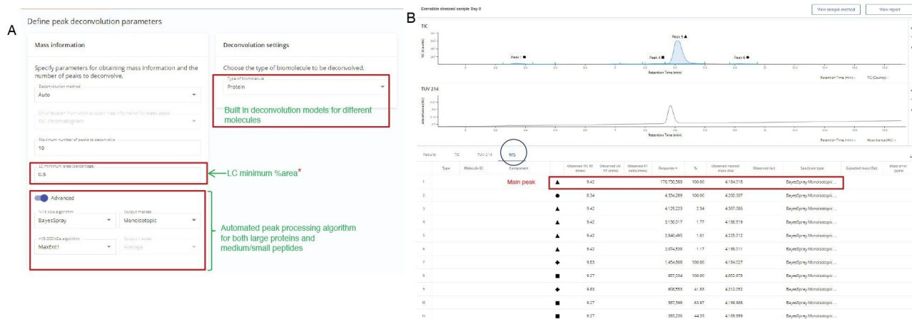
Figure 2. A) Intact Mass App processes data using built-in peak deconvolution algorithms. The BayesSpray algorithm was used with deconvolution settings for proteins for Exenatide. B) The untargeted analysis shows the neutral masses of compounds calculated based on the MS data. Each MS data point is marked by a symbol that refers to a chromatographically separated peak shown on the TIC above. Each mass shows a retention time that facilitates the identification of the chromatographic peak. The main peak 5 with 4184.018 Da is the most abundant component (API).
