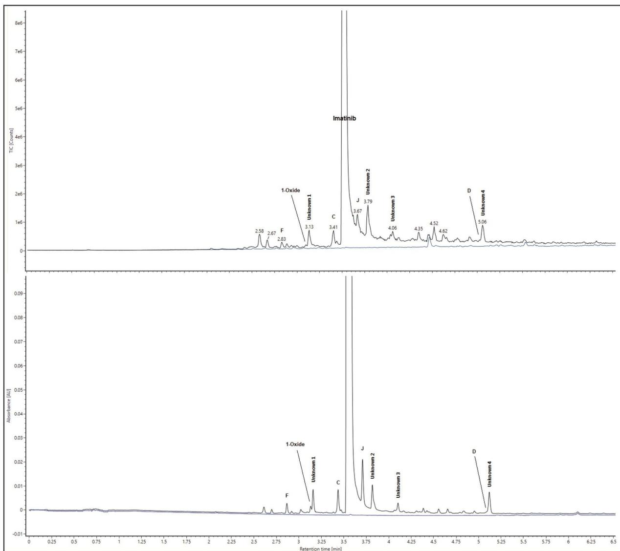
Figure 1. Separation of imatinib and related impurities with MS-compatible mobile phases and an ACQUITY Premier CSH Phenyl-Hexyl column (2.1 mm x 100 mm C<sub>18</sub> 1.7 μm, 130 Å). Detection: 267 nm. Flow rate: 0.4 mL/min. Gradient: 0.5% B to 100% B in 10 minutes with a linear gradient. Upper chart: TIC traces of imatinib and methanol blank. Lower chart: UV 267 nm traces of imatinib and methanol blank.
