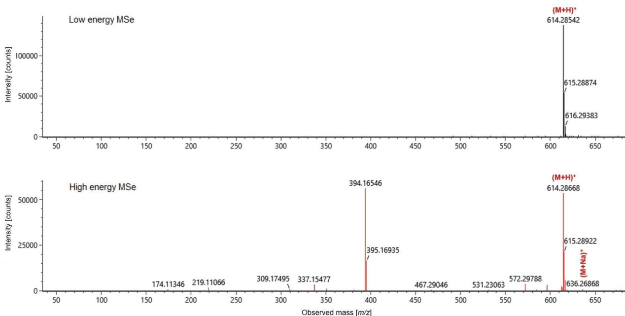
Figure 2. HDMS<sup>E</sup> fragmentation spectra of the ions of interest ( $m/z$  614.28) in positive mode.
