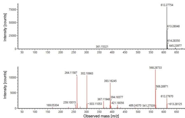
MSe spectra of Imatinib Benzoic Acid standard
