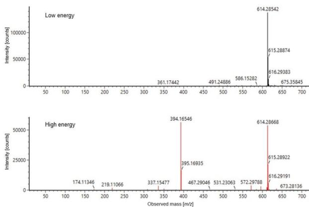
MSe spectra of Imatinib Benzoic Acid standard
