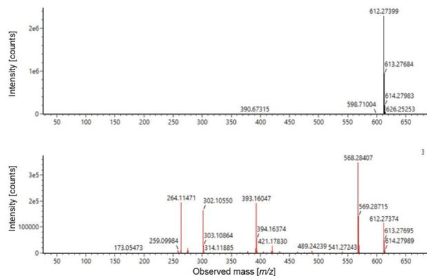
Figure 9. Comparison of negative ion mode HDMS<sup>E</sup> spectra of imatinib benzoic acid and Unknown 3.
